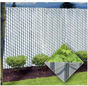
Fin2000® Pre-Woven is a premium style slat with innovative "fins" that give extra screening and security. This slat is mechanically inserted into the chain link wire fabric during the weaving process. Once inserted, the wire is finished above and below the slat (either bow-knuckled or knuckle-over).
