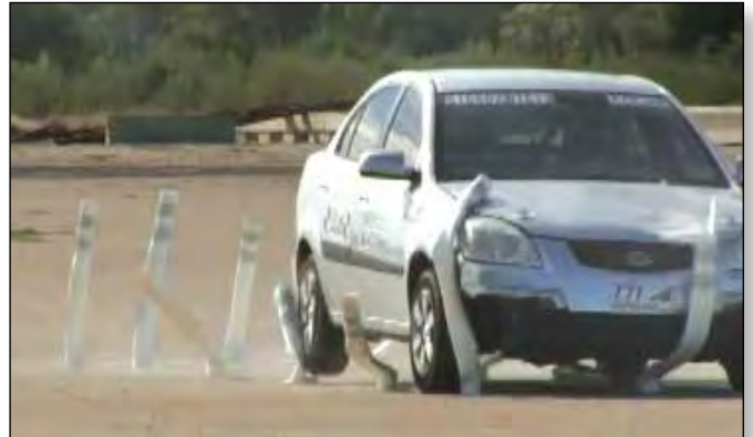
City Posts rebound back to their original position, even after more than 100 high-speed hits on the TTI Test Deck
