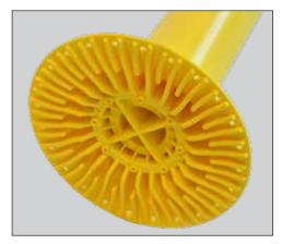
The base of the City Post GD is just 8" wide, fitting perfectly between the standard paint markings on the roadway. The unique pinwheel design maximizes surface area for better adhesion of the epoxy.
