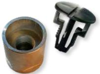
The anchor cup allows for easy removal of the channelizer if needed. Anchor cups are mounted below the roadway grade and feature an optional removable cap. The caps keep debris out of the cup when posts are removed for winter plowing operations, or in areas where parades or festivals take place. This post is the ideal answer for installations where occasional removal is required or desirable.
